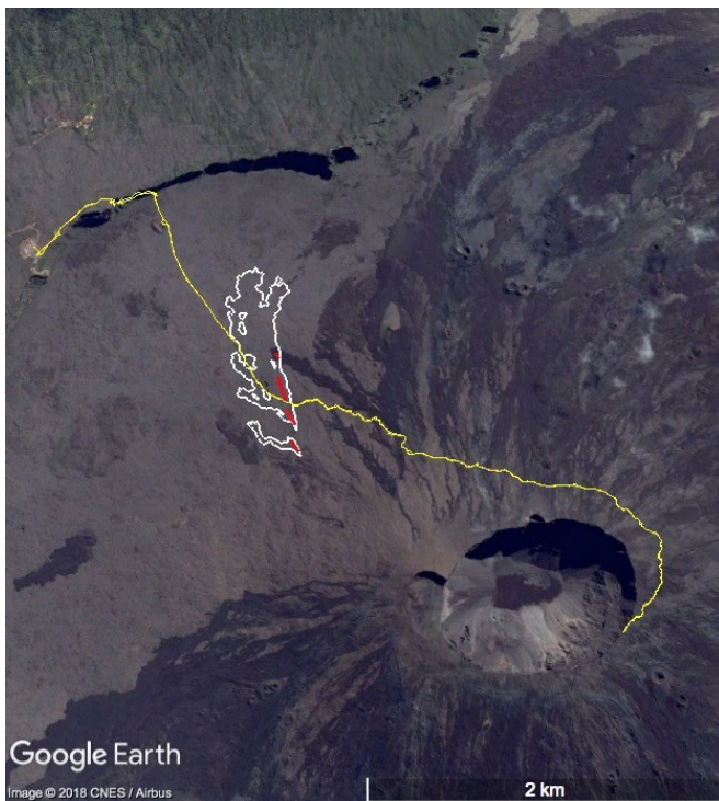
Figure 15: Final map of the lava flows emitted during the July 13, 2018 eruption. This map was produced based on aerial and ground-based photographs processed by means of stereophotogrammetry. Lava flow outlines are shown in white, eruptive fissures in red and the hiking trail to the summit in yellow.
